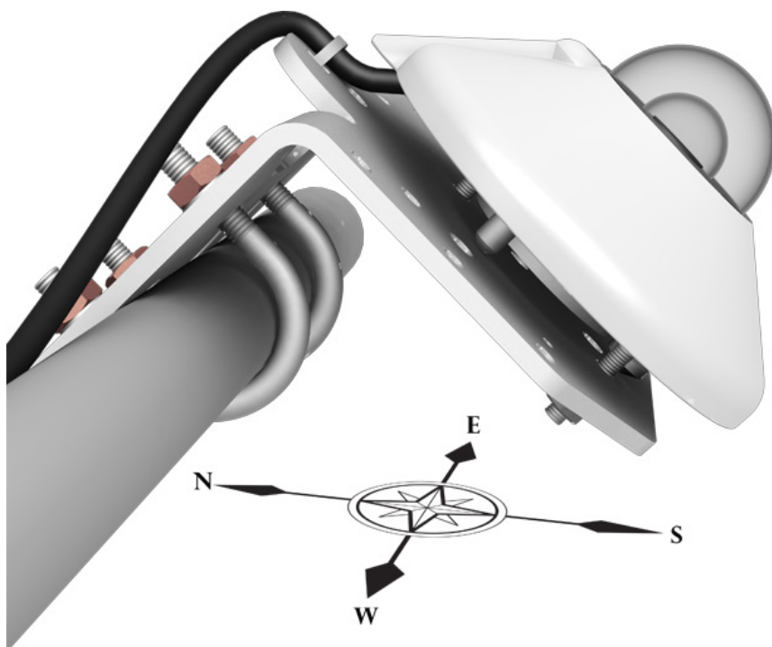
FIGURE 7-4. Pyranometer mounted at an angle for the Southern Hemisphere
