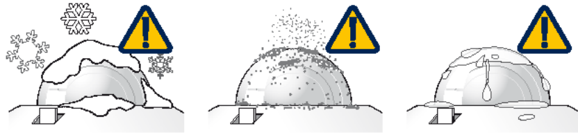
FIGURE 8-1. Reading is reduced if dome is not dry or clean
